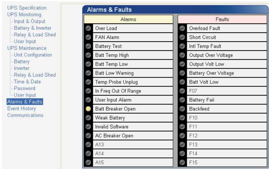
Figure 44 — Alpha UPS Monitor: UPS Alarms & Faults screen
