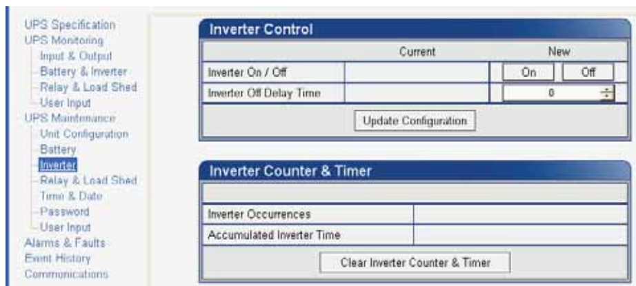
Figure 24 — UPS Maintenance: Inverter screen
