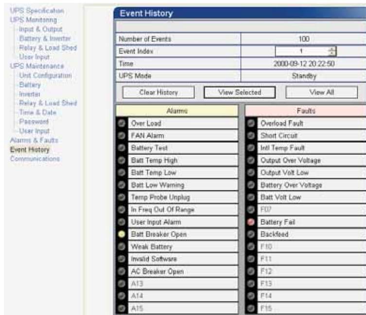
Figure 43 — Alpha UPS Monitor: UPS Event History screen
