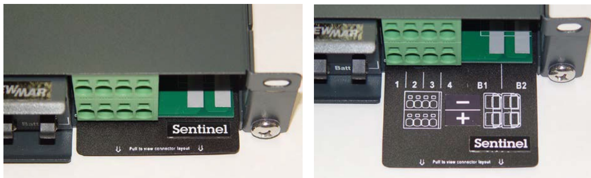
Fig 3 & 4, DC Connector detail and pullout guide
