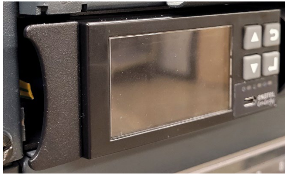
Fig 6. For removal, pull monitor forward to release the ball catch
