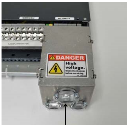
AC Junction Box
