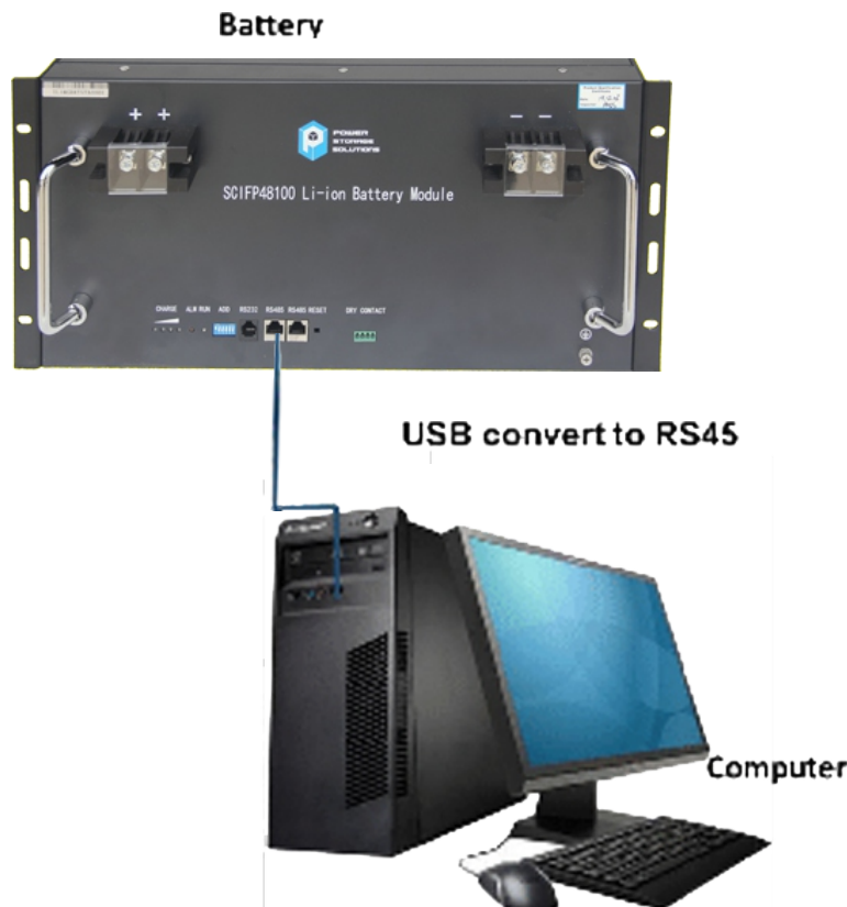
Figure 5-3: Communication Cable Connections between Battery and Computer
