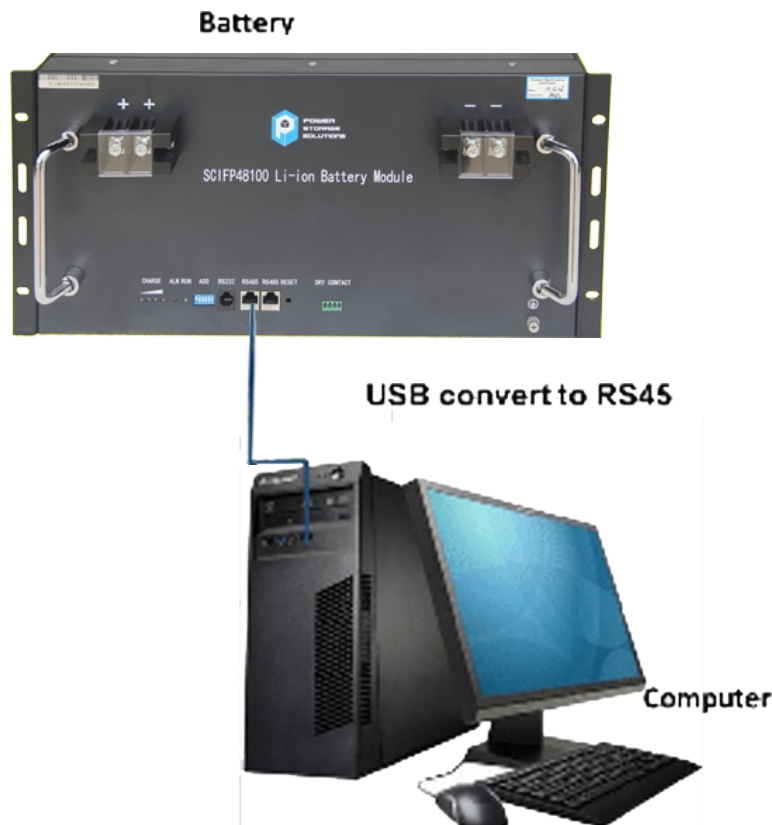
Figure 5-3: Communication Cable Connections between Battery and Computer
