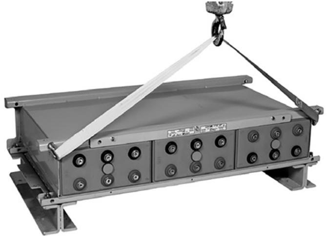
MODULE WITH BASE ASSEMBLY AFTER TIP-OVER Figure 13
