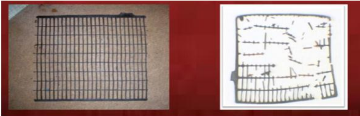
Comparison of TPPL grid and lead calcium alloy grid after elevated temperature float life testing – Batteries were torn down after elevated temperature float life testing and positive electrodes were removed. Positive Active Material (PAM) was carefully removed and the remaining grid was photographed. The TPPL positive grid on the left, is fully intact with minimal loss of grid mass. The conventional lead calcium grid (shown on the right) is no longer intact, having lost a large portion of its material through grid corrosion.
