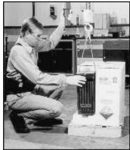
FIGURE 1.4.2 - Use of lifting sling and spreader board
