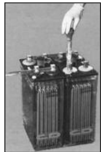
FIGURE 2.6.1 - Taking a hydrometer reading
